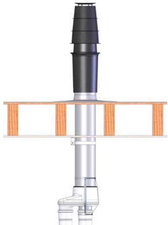
Typical flat roof situation
